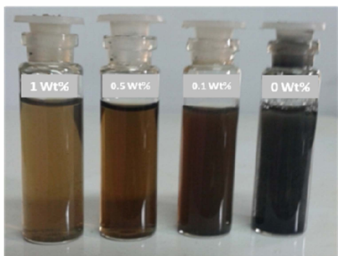
Fig 2 Photo of PbS nanoparticles capped with different concentration of 2-Mercaptoethanol
